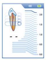
Further progression of the file in the canal is shown both by the cursor on the tooth icon and by the numerical value on the graphical scale (which does not represent length in millimeters). Detect™ emits audible information of file progression via a series of progressive rate beeps.
