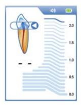
A blinking cursor and no sound signal indicate a faulty connection. Check your connections, clean your hook connection, moisten the canal, if necessary, and start again.
